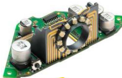
Lighting System for Security Camera v300 ws (HARTING Mitronics for SICK, LCP LDS
